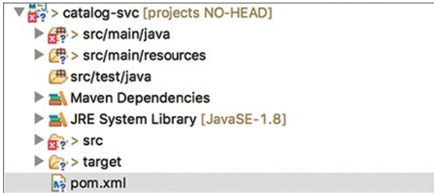
Figure 12.3 Structure for a microservice in Eclipse
