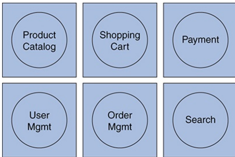
Figure 1.6 E-commerce system components broken down into standalone microservices
